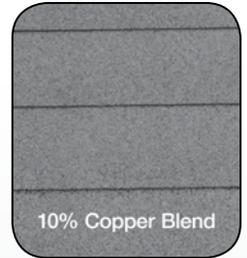
Grey scale images showing black streaks caused by algae growth on shingles exposed in Houston, TX for 5 years. Shingles with low blend percentages show significant discoloration already.
