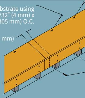
Appropriate fastener for substrate on every vertical "Z" bracket through vertical "Z" brackets and backer
