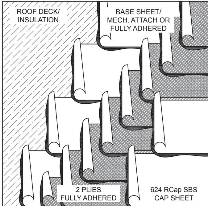
Four-ply, hot mopped, built-up roofing system with conventional fiber-glass base/ply sheets and a highly-reflective, factory coated SBS cap sheet installed over an approved roof deck.
