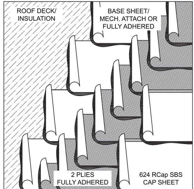
Four-ply, hot mopped, modified built-up roofing system with SBS fiberglass base/ply sheets and a highly-reflective, factory coated SBS cap sheet installed over an approved roof deck.
