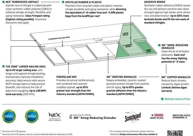
Test Compliance - ASTM D7158 Class H, ASTM D3462, ASTM D3161 Class F, ASTM D3018 Type I, ASTM E108 Class A Fire Rating, UL 2218 Class 4, CSA A123.5, ICC Approval - ESR-3150, and ICC-ES AC438.
